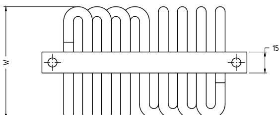
The number of wire rope loops can be less than 8, f.inst. 4 or 6, whereat the load range is correspondingly reduced.
