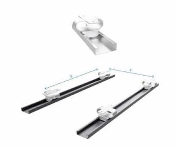
Figure 1: The VT-ACC system. In the tests the hangers were mounted with c/c 800 mm (G) and the profiles were mounted with c/c 600 mm (P).
