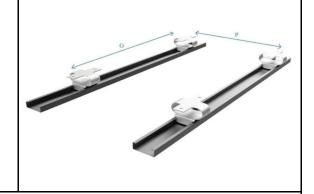
Test sample, reduction of impact noise
