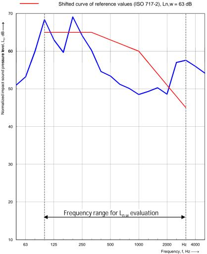
Test sample, Lnw = 63 dB
