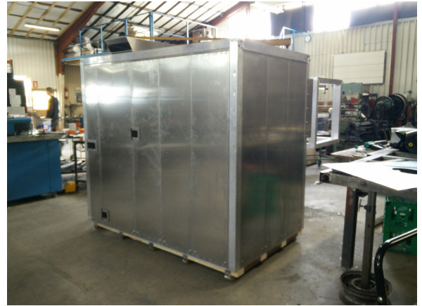
Assembled offshore enclosure
