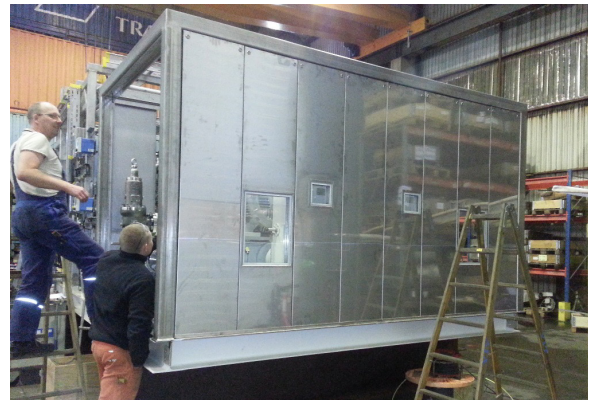
Test assembly of offshore enclosure
