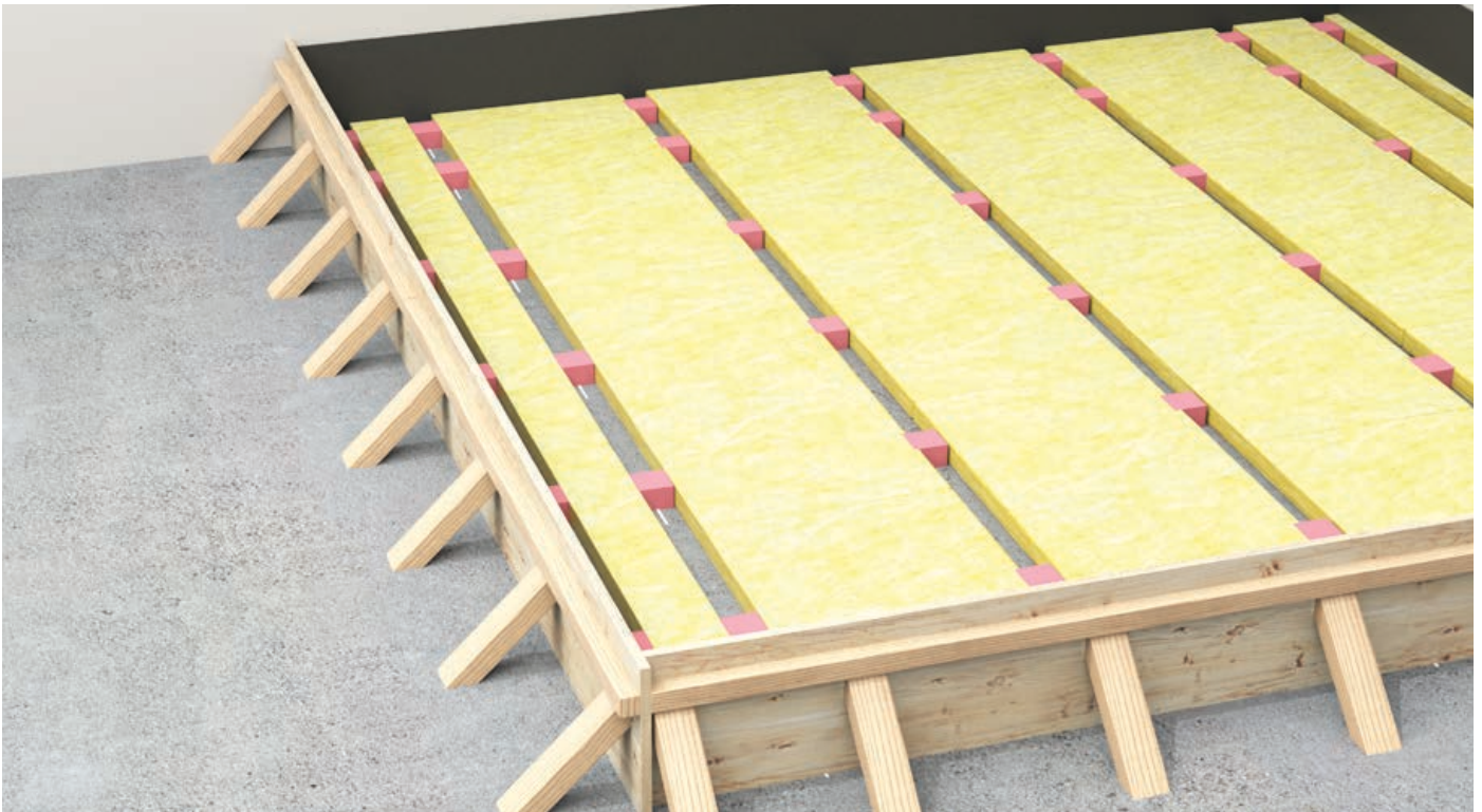
Image C-1: Mineral wool between the rows of Regufoam or spring isolators.
