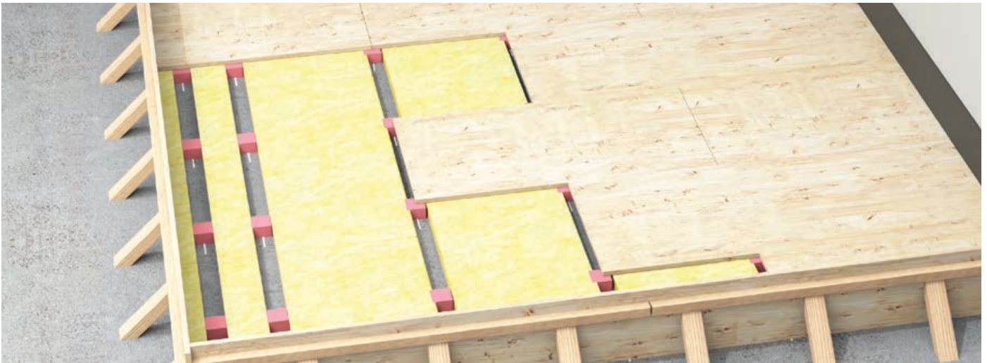
Image D-1: Mineral wool between the rows of Regufoam or spring isolators.
